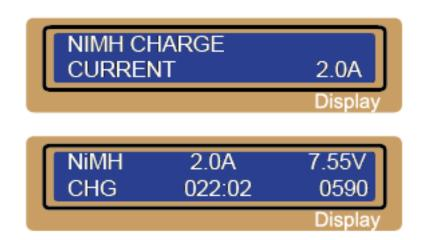
After completion of the chosen charging function, the following information screen is displayed. You will be informed of the charge current, terminal voltage, charging time and the charged capacity.
