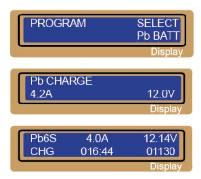
After end of charge, some charging data (Battery voltage, maximum charge current, duration of charging, charged capacity) is displayed on the LCD.
