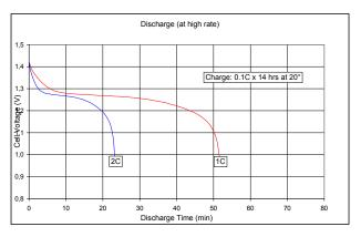
Delivered capacity is dependent on the applied load, operating temperature and cut-off voltage.. Data in this specification is subject to change without notice. Rev. 10/2014.
